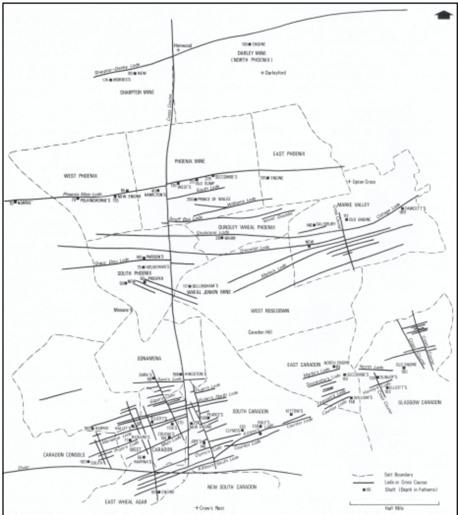
Figure 2 - Principal Lodes, Setts and Shafts of Caradon and Phoenix Mining Area.
