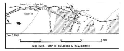
resembled a fracture zone rather than a single fault line and the mineralised area may have been as wide as sixty feet in places. The vein filling is a fault breccia cemented by quartz with some calcite, while at the Esgair Fraith end of the sett
