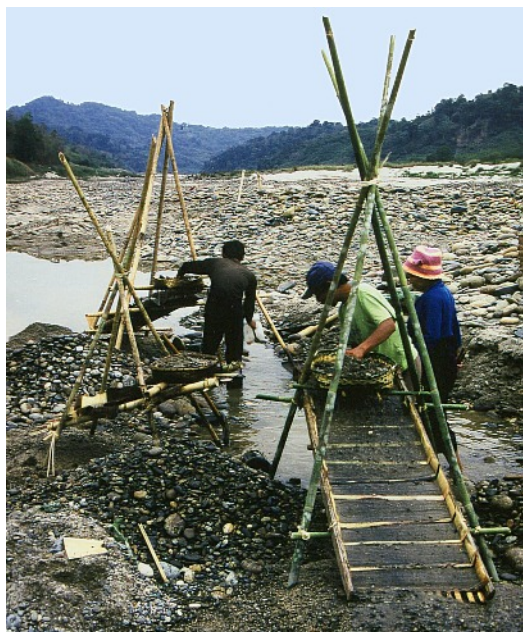
Fig 2 Using a trestle containing a sluice box, the prospector washes his gravels through a basket
