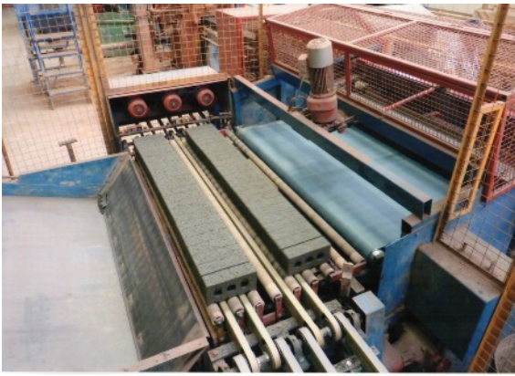
Photo:- Brick-cutter area, where the extruded lengths are cut to brick size
