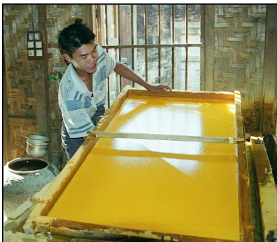
Fig 1 A Burmese boy making paper from bamboo. This paper does not adhere to gold and when used as interleaves, it protects the gold-leaf offered for sale.
