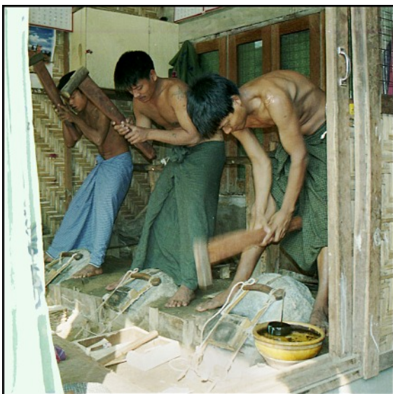
Fig 2 Preparing gold leaf from small 2oz billets of gold by strenuous hammering. The men must make 120 strokes before the special clock (a 'clepsydra', which is made from a punctured coconut shell) sinks in the bowl of water
