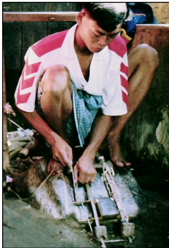
Fig 3 The extruder-device that controls the gold emanating from the gold billet during the hammering stage
