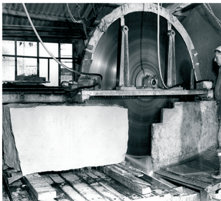
1918 Anderson Grice three meter primary saw installed to cut war graves. Originally this machine was steam driven
