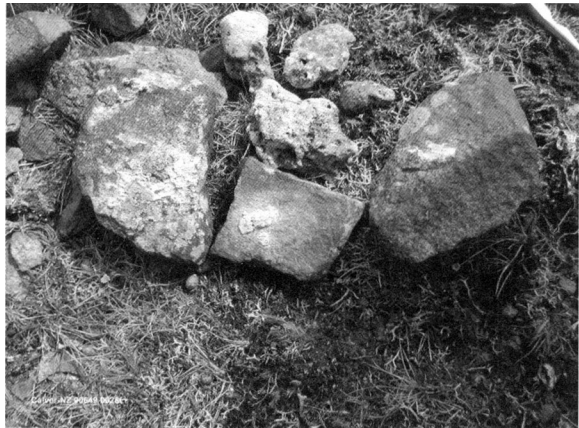
Plate 4. Splashes of lead silicate slag and lead on stone, typical of Type A slag and pieces of grey barytes slags typical of Type B
