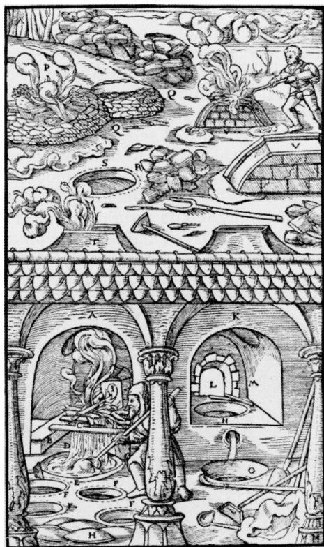
A—FURNACE OF THE CARNI. B—LOW WALL. C—WOOD. D—ORE DRIPPING LEAD. E—LARGE CRUCIBLE. F—MOULDS. G—LADLE. H—SLABS OF LEAD. I—RECTANGULAR HOLE AT THE BACK OF THE FURNACE. K—SAXON FURNACE. L—OPENING IN THE BACK OF THE FURNACE. M—WOOD. N—UPPER CRUCIBLE. O—DIPPING-POT. P—WESTPHALIAN METHOD OF MELTING. Q—HEAPS OF CHARCOAL. R—STRAW. S—WIDE SLABS. T—CRUCIBLES. V—POLISH HEARTH.
