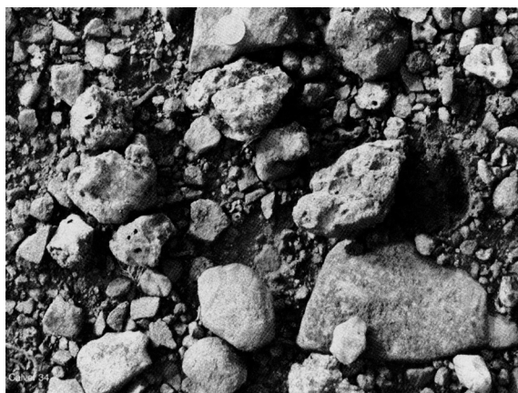
Plate 9. Typical Type C slags at site C17. They are characterized by their grey irregular exterior; sometimes showing flow marks and gas vesicles.
