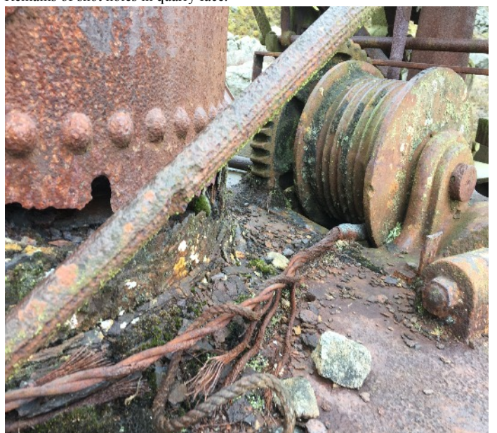
Boom winch with rope and hemp clearly visible.
