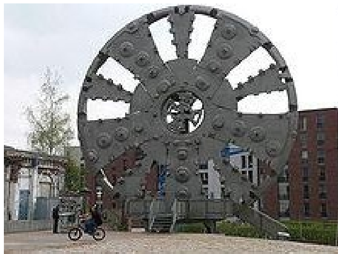
The cutting shield used at the head of a TBM.
