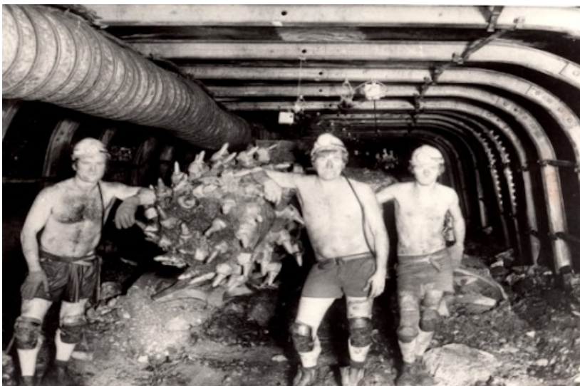
September 1984. Dosco LH1300 and team. Driving K25 main gate in the East side. Blackshale seam.
